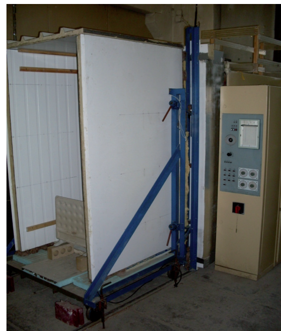
Figure 4 - Testing procedure of facade heat insulation structures with rendering for resistance to climatic influence
